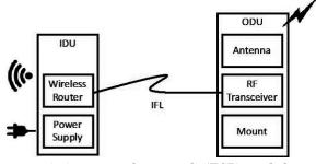
of transmission control protocol (TCP) and hypertext transfer protocol (HTTP)), as well as certain signal conversion, modulation, and amplification functions. The IDU also incorporates a Wi-Fi router that can be accessed by end users (and their communications devices) in the same manner as other Wi-Fi routers. The IDU interfaces with the ODU through the inter-facility link (described below).60
